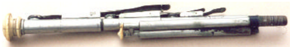
Figure 13 'Scott' double-bass regulator
